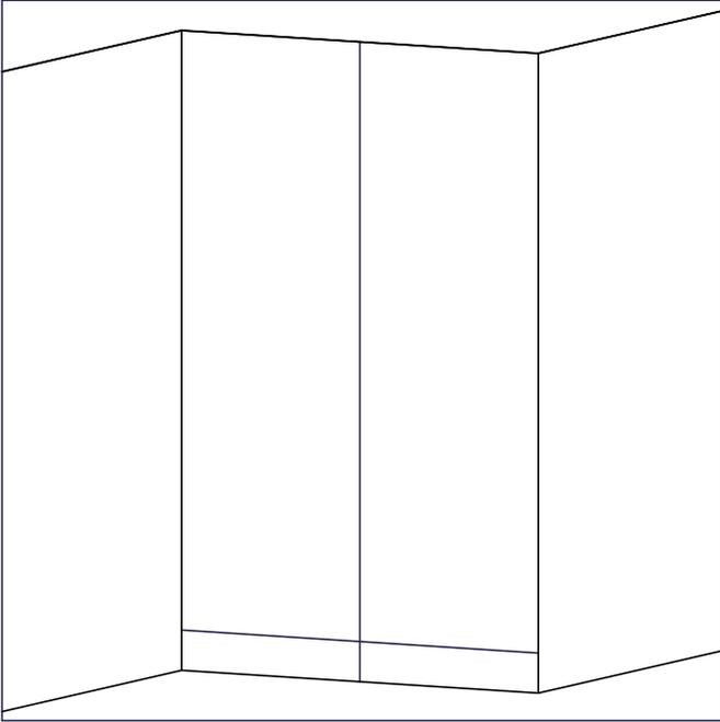
1) Draw a vertical line at the midpoint of the wall. If using an odd # of profiles, measure 2" to the left or right of the center line and begin there. Doing this will offset this first profile so each side is symmetrical.
