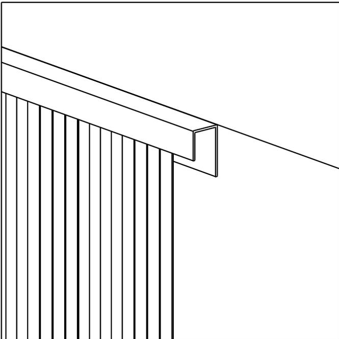
3) It is recommended to add a channel to the top of the wall to hide the cut ends. This could help ease installation since this method would allow rough cut sizes instead of having to precisely cut each piece if you have an uneven wall height.
