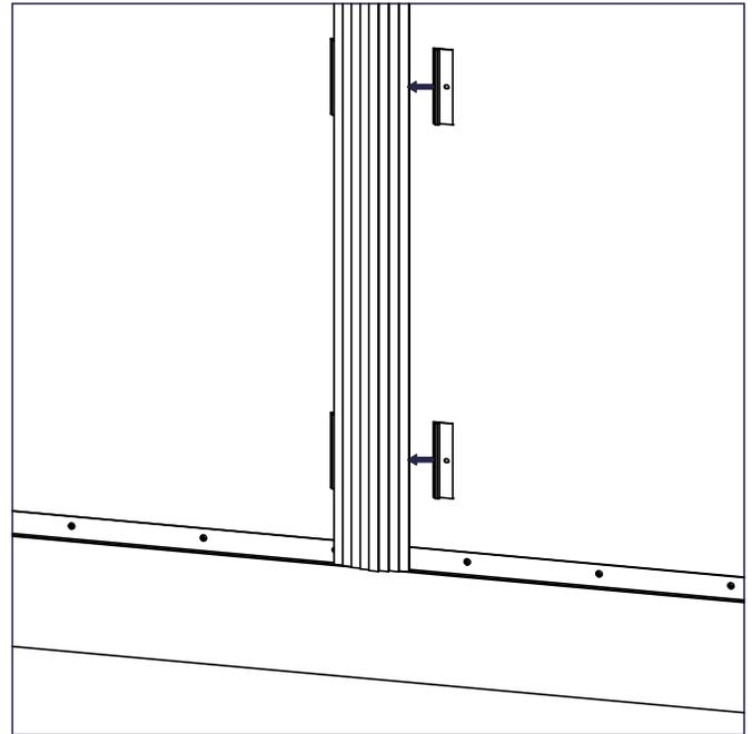
6) Secure the AXIA profile in place using Intermediate connectors. Make sure there is a tight fit between the connector and the profile before fastening the connector to the wall.
