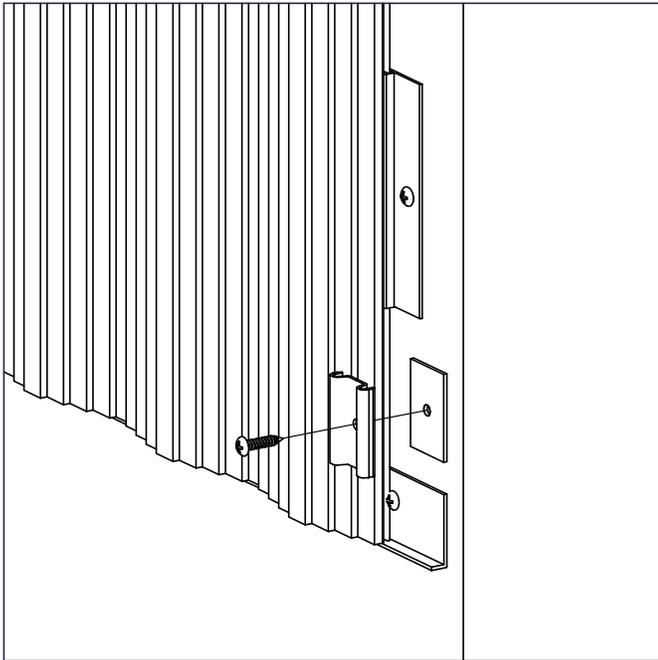
9) Fill the open gap on each end using Stylmark TrimMaker. Install plastic base clips and spacers 3-4" inches from each end and approximately 30-36" apart.
