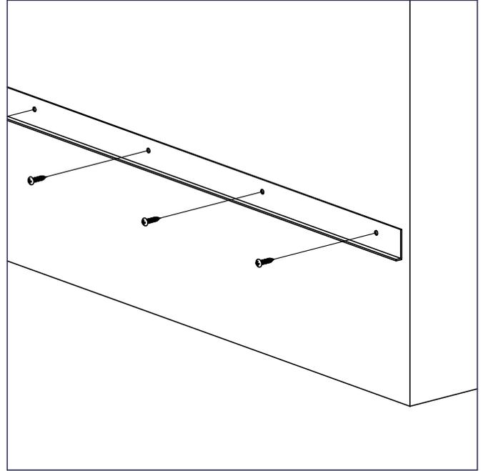
2) If the AXIA profiles will not rest directly on the floor or a baseboard, install an angle (or similar) to support the AXIA profiles.
