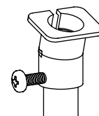
Part #510622 Rigid Connector 1/2" Downtube
